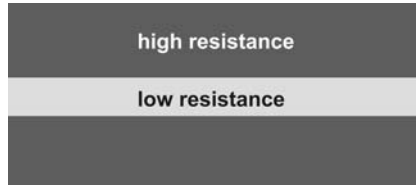
FIGURE 5.1. A surface with a central strip having a low resistance to fluid flow surrounded by strips with high resistance to fluid flow
