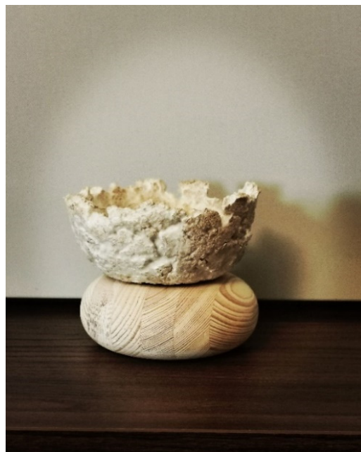
Figure 13. Finished object: mycelium-based bowl fixed to the rough-timber torus-shape base (design and photo: A. Bonenberg).
