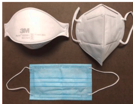
Fig. 1. Standard face mask 3MN95 (Aura TC-84A-8590) (left), KN95 (right) and surgical (down) used in this study.
