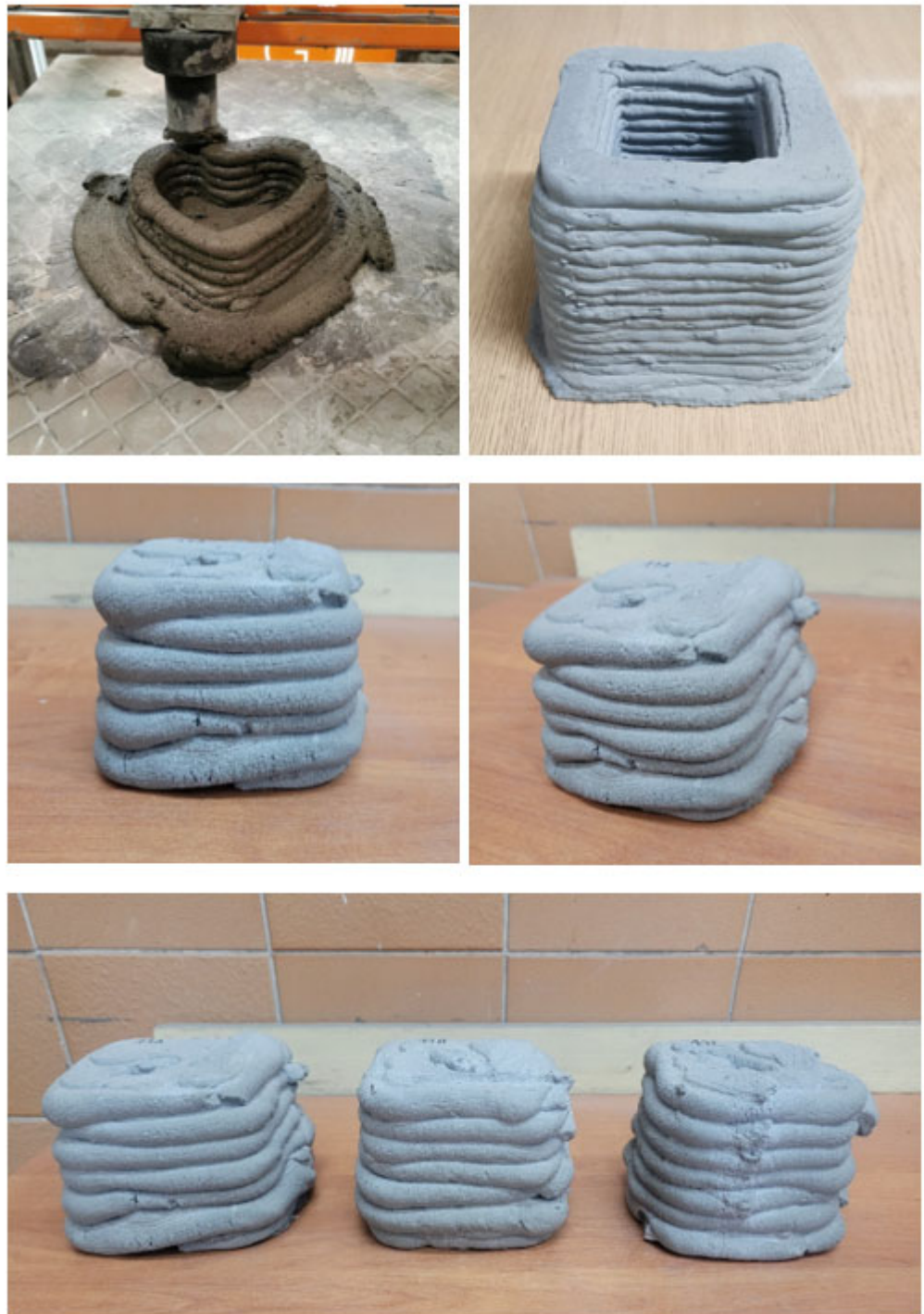
Figure 8. Sample printouts from a 3D printer.
