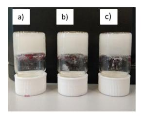
**Figure 1.** Representative results obtained from inverted vial tests. (a) PVA/CS 2, (b) PVA/CS/BG 2/0.5 and (c) PVA/CS/BG 2/1.5 hydrogels.
