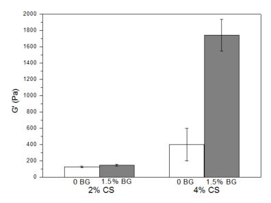
**Figure 4.** Elastic modulus at frequency = 1 Hz for PVA/CS 2, PVA/CS/BG 2/1.5, PVA/CS 4 and PVA/CS/BG 4/1.5.
