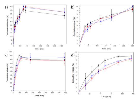
**Figure 7.** Drug release profile of (a) and (b) PVA/CS 2 ( $\blacksquare$ ), PVA/CS/BG 2/0.5 ( $\bullet$ ) and PVA/CS/BG 2/1.5 ( $\blacktriangle$ ) and (c) and (d) PVA/CS 4 ( $\blacksquare$ ), PVA/CS/BG 4/0.5 ( $\bullet$ ) and PVA/CS/BG 4/1.5 ( $\blacktriangle$ ) Samples immersed in 100 mL of PBS (pH 7.4) at 37 °C for 5 h.
