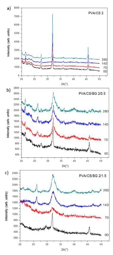
**Figure 6.** XRD patterns of hydrogels after immersion in SBF for different times. (a) PVA/CS 2, (b) PVA/CS/BG 2/0.5 and (c) PVA/CS/BG 2/1.5.
