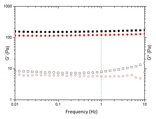
**Figure 3.** Elastic modulus (**closed symbols**) and loss modulus (**open symbols**) as a function of frequency of PVA/CS 2 ( $\bullet$ ) and PVA/CS/BG 2/1.5 ( $\blacksquare$ ).
