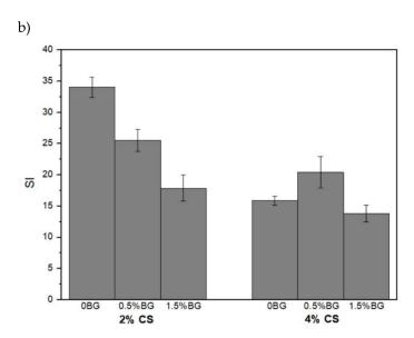
**Figure 2.** (a) Equilibrium water content (EWC) and (b) swelling index (SI) of the hydrogels immersed in 50 mL distilled water at room temperature for 2 h.
