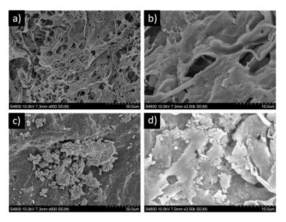
**Figure 5.** Scanning electron micrographs of PVA/CS 2 at day 0. (a) Magnification  $\times$ 600, (b) magnification  $\times$ 3500) and PVA/CS/BG 2/1.5 after 28 days submerged in SBF, (c) magnification  $\times$ 600 and (d) magnification  $\times$ 3500).
