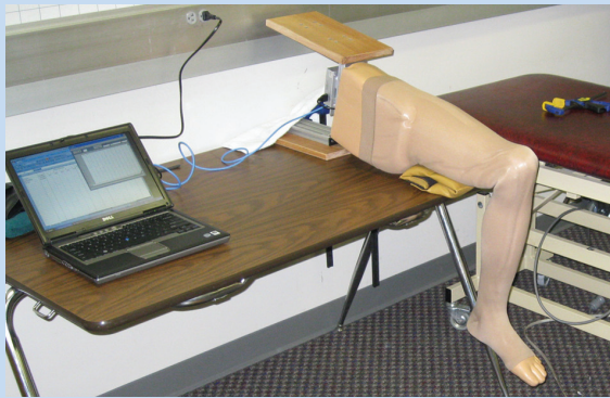
Figure 1. The instrumented test leg used for torque data collection.
