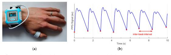
**Figure 1.** Acquiring photoplethysmography (PPG) signals in daily living: (a) the SmartCare wristworn pulse oximeter used to record the PPG at the thumb; (b) a sample PPG signal (in arbitrary units), with red circles indicating individual heartbeats.
