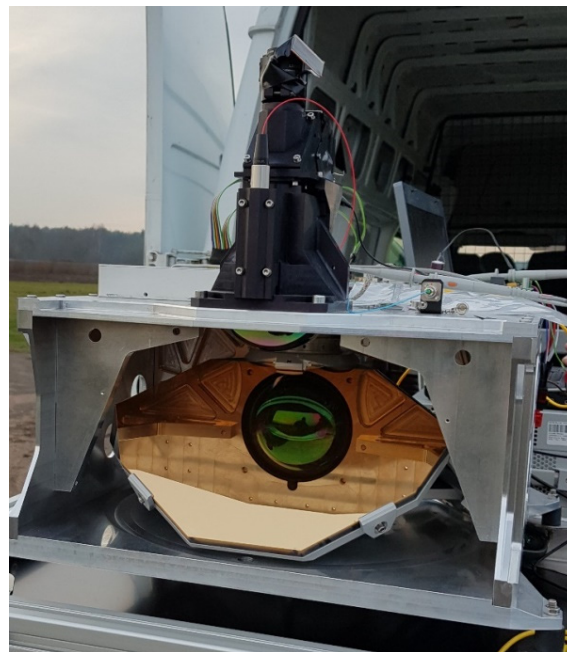
Figure 4. Photography of the constructed anti-drone laser scanner prototype.
