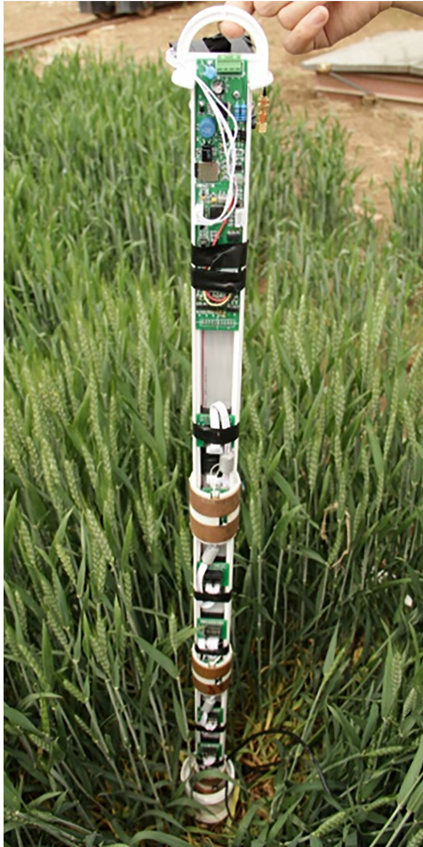
Fig 5. Field ring probe of soil freezing and thawing sensor [41].
