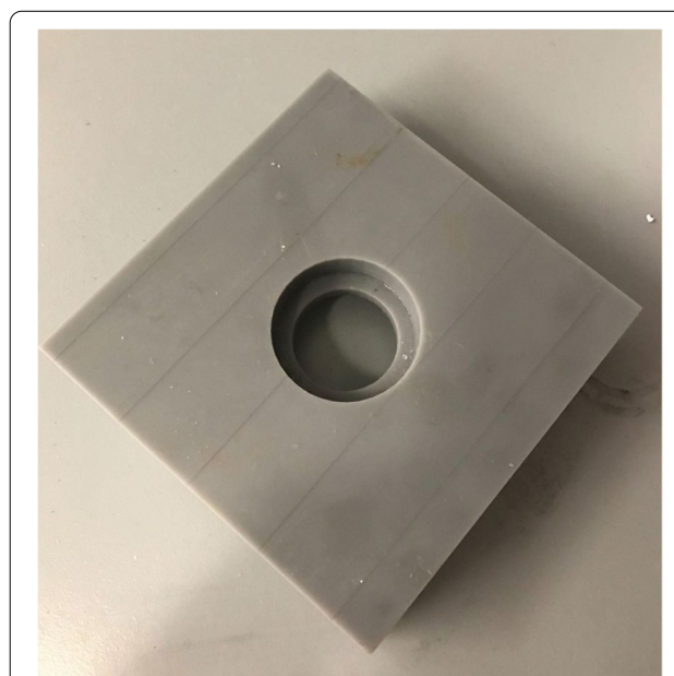
Fig. 6 The 3D printed jig used to position the filled molds for testing with the Instron
