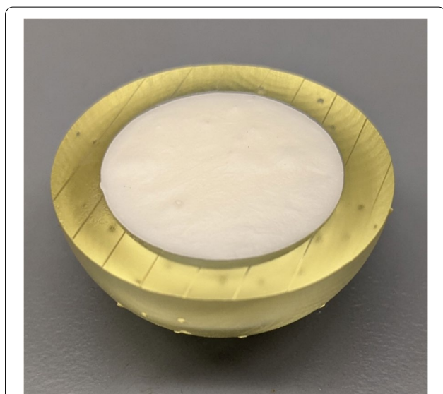
Fig. 5 A hemispherical mold filled with bone cement
