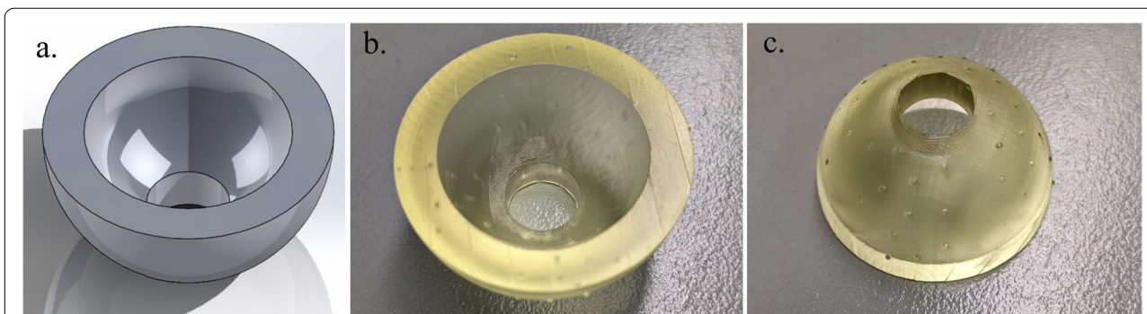
Fig. 2 The SolidWorks model of the hemispherical mold (a). Concave surface of mold (b). Back of mold (c). The inner diameter of the mold is 2.5 cm with a height of 1.25 cm, and the outer diameter is 3.5 cm with a height of 1.75 cm
