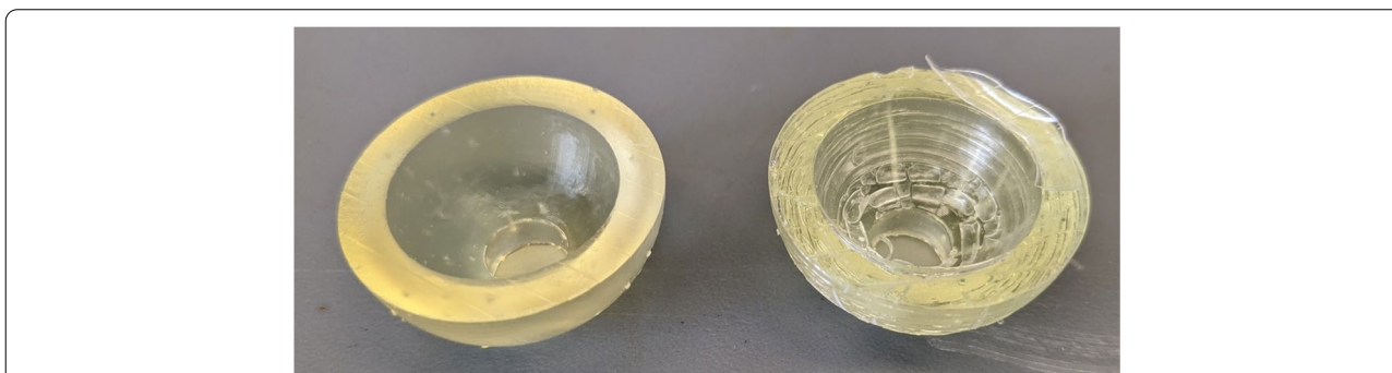
Fig. 3 Normal mold (left) next to a mold deformed by the autoclave cycle due to remaining IPA from the wash step that did not evaporate before the post-cure step (right)
