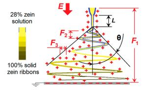
**Figure 9.** A diagram showing the formation mechanism of electrospun nanoribbons through the modified coaxial electrospinning.
