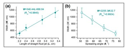
**Figure 8.** The correlations between the width of electrospun zein nanoribbons and: (a) The length of the straight fluid jet; and (b) the spreading angle of the unstable zone.
