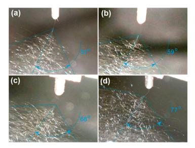
**Figure 4.** The changes of spreading angle and the length of straight fluid jet with the increase of LiCl in the sheath solution (mg/mL): (a) 0; (b) 5; (c) 10; (d) 20.
