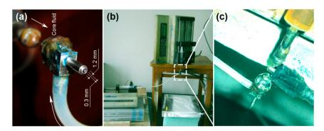
**Figure 3.** The apparatus used for modified coaxial electrospinning: (a) The home-made concentration spinneret; (b) the arrangement of apparatus; and (c) the connection of the power supply and working fluids with the spinneret.
