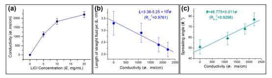
**Figure 6.** The influence of the sheath fluid conductivity on the behavior of the working fluids: (a) The relationship between LiCl concentration and solution conductivity; (b) the decrease in the length of the straight fluid jet with an increase of conductivity; (c) the increase of spreading angle with rising conductivity.
