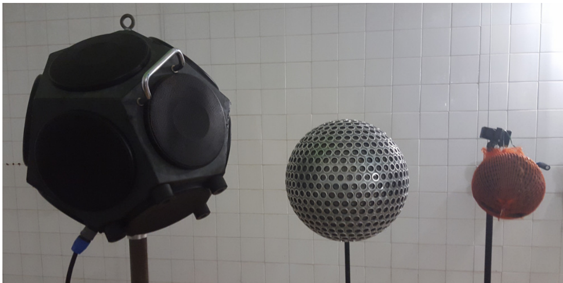
Figure 1. From left to right, commercial dodecahedral loudspeaker, new OPL and old OPL. The sound sources have, respectively, a diameter of 0.4 m, 0.25 m and 0.12 m.
