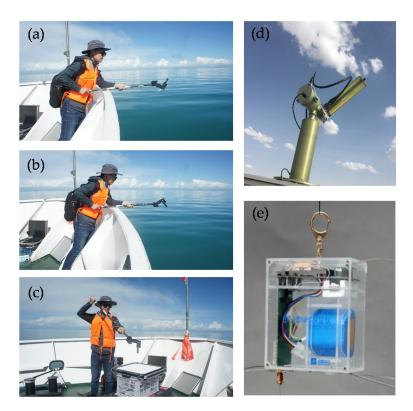
**Figure 5.** Observation equipment used in the experiment: (a–c) an ASD FieldSpec4 spectrometer for acquiring water surface parameters; (d) a CE-318 automated sun photometer for measuring atmospheric parameters; (e) a GPS radiosonde for obtaining PTU.
