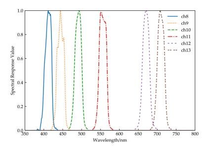
Figure 1. Spectral response function of the FY-3D/MERSI-II.
