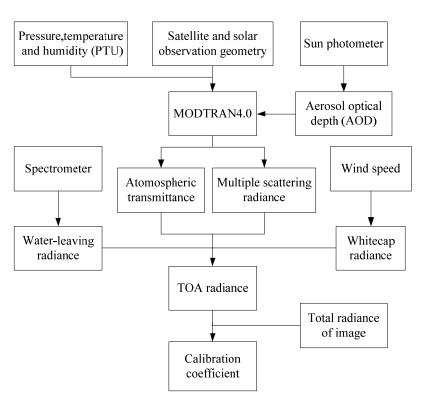
Figure 2. Flowchart of vicarious calibration method.
