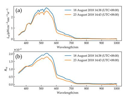
Figure 6. (a) Water-leaving radiance; (b) remote sensing reflectance.
