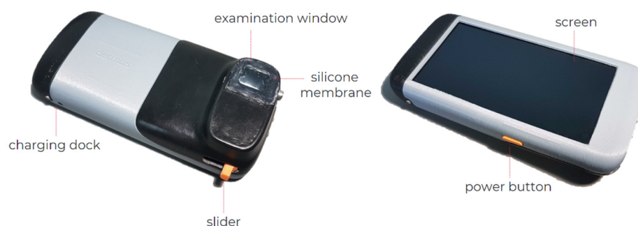
Figure 1. The Dermus SkinScanner device with its main components, including an examination window with a silicone membrane cover, screen, charging dock, power button and slider (for mechanical scanning).
