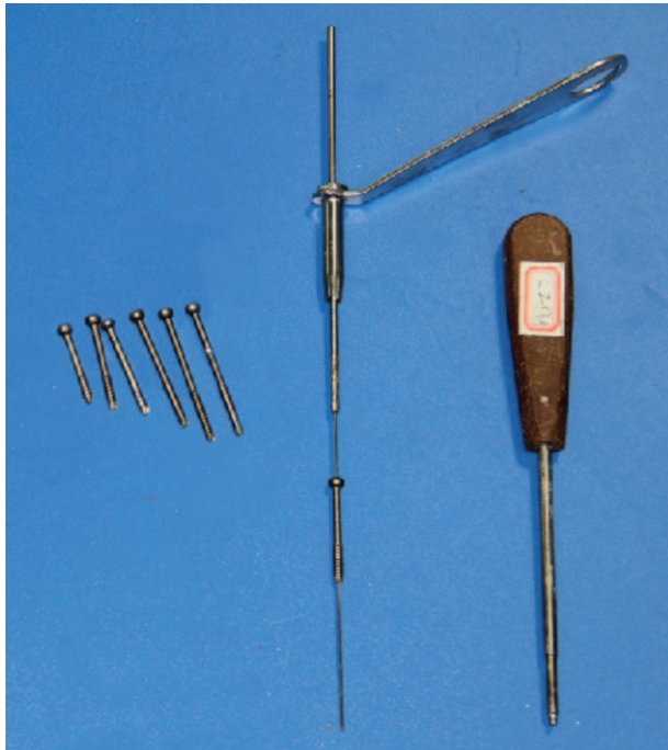
FIGURE 3. Photograph showing the system of tools to facilitate insertion of screw.
