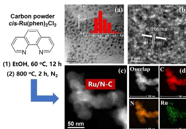
**Figure 9.** Procedure for the synthesis of Ru/M-C: a) TEM image, b) HRTEM image, c) HAADF-STEM image, and d) STEM-EDS elemental mappings of Ru/N-C. Reproduced from with permission from ref.[45]. Copyright 2018 Wiley-VCH.
