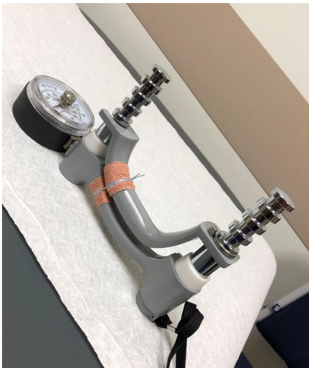
Figure 1 Jamar Hydraulic Hand Dynamometer with number 5 FiberWire demonstrating compression testing.
