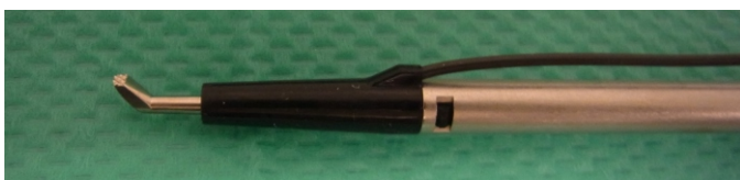
Figure 6: An image of an ultrasonic bone curette. The tip of an ultrasonic bone curette was developed to be bent moderately to use easily under a microendoscope with the property of its 25° oblique view.
