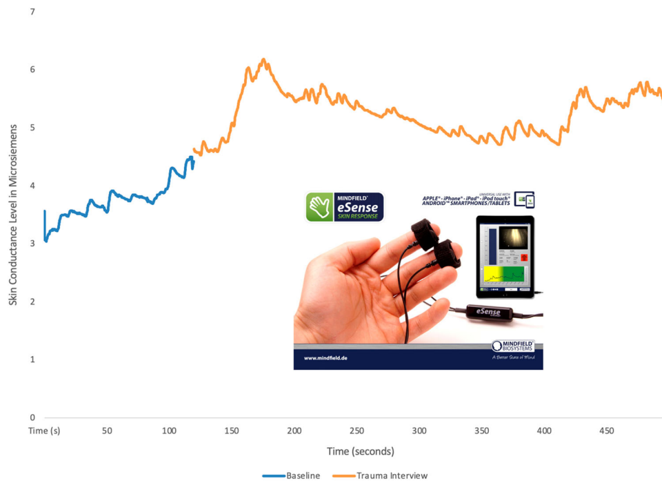
Figure 1. Mobile continuous recording of electrodermal activity using the Mindfield eSense set-up from n = 1 participant. This set-up requires one set of electrodes which are placed on the middle phalanges of the index and middle finger. The electrodes connect to any smart device running the eSense app. A two-minute baseline is first obtained, followed by the trauma interview. The baseline recording and trauma recording from the entire duration of the HTQ administration (trauma interview) is depicted.
