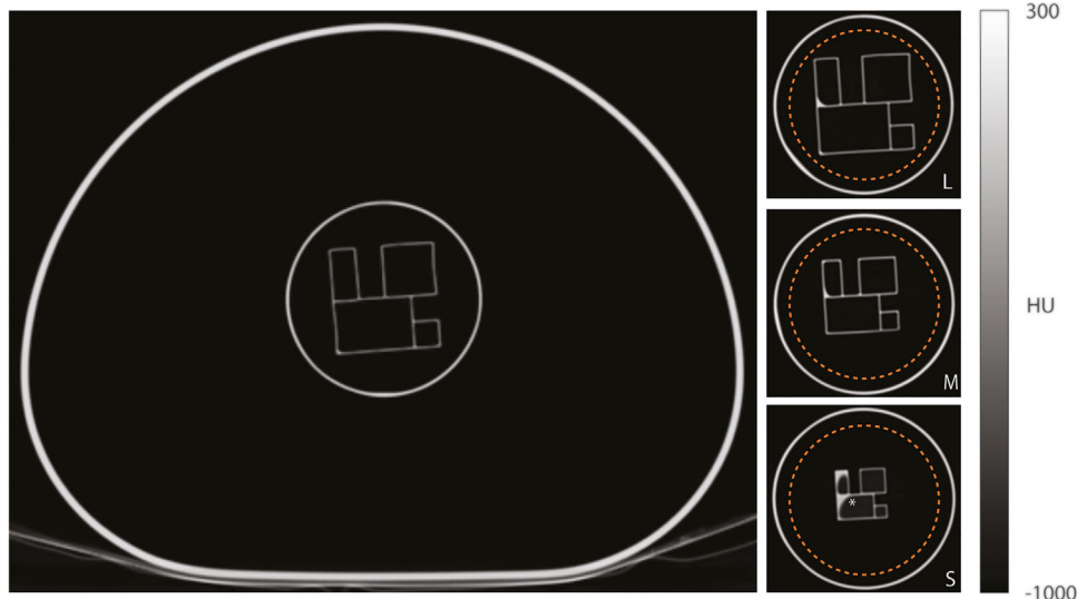
FIGURE 2 High-resolution computed tomography (CT) images of the heterogeneity phantom. The orange dashed lines represent the volume of interests (VOIs) of the detailed images of the large (L), medium (M), and small (S) inserts. Note that in the small-sized insert, some residual water from the leakage test is present in this image(*)
