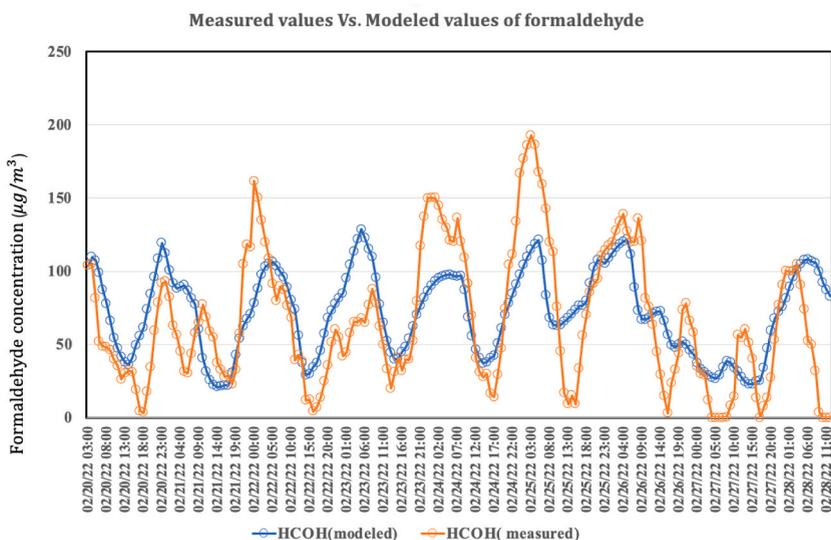
Fig. 8. Comparison of Formaldehyde values simulated by CONTAM with measured data.
