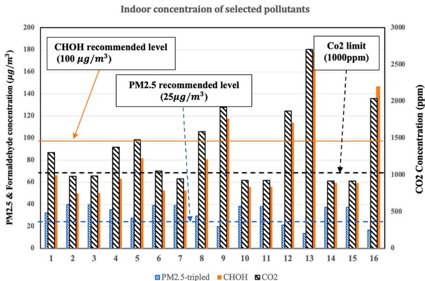
**Fig. 9.** The concentration of selected pollutants in the indoor environment for combined scenarios)In the condition of critical levels of outdoor PM2.5).
