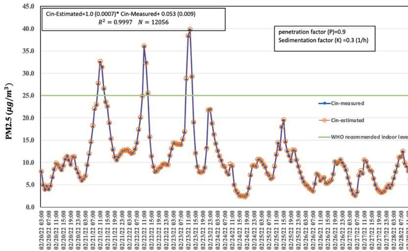
Fig. 4. Estimated and measured values of indoor PM2.5 concentration and their regression relationship. \*(The numbers in parentheses are the standard error of the model coefficients).
