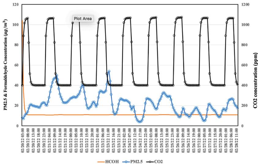
Fig. 11. Concentration of PM2.5 and formaldehyde if using a fresh air supply system with particle filter with 70% efficiency.
