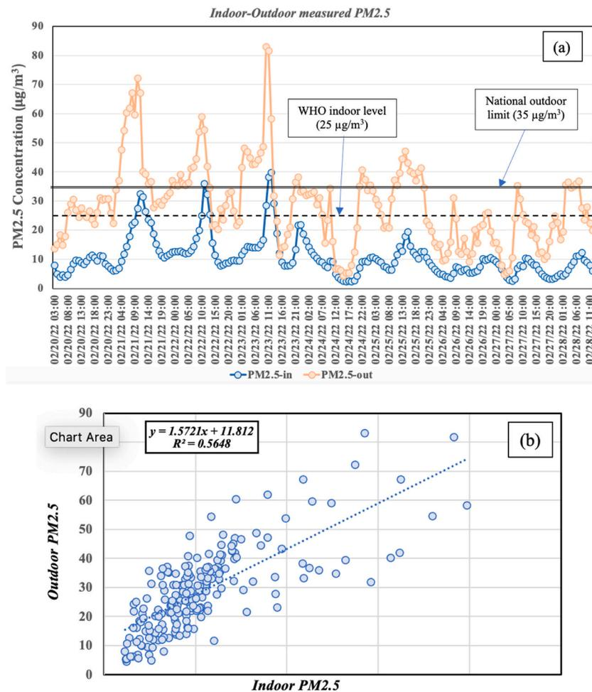
Fig. 5. Indoor and outdoor PM2.5 mass concentration (a) and correlation (b) for the measurement period (February 20 to 28).
