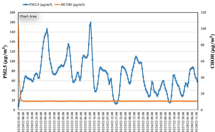
**Fig. 10.** Concentration of PM2.5 and formaldehyde in case of using a fresh air supply system without particle filtration.
