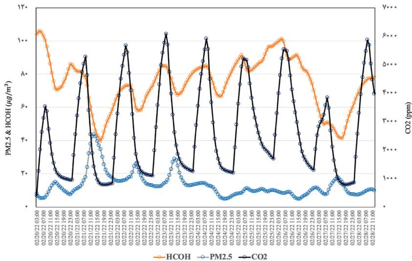
Fig. 12. Concentration of PM2.5 and formaldehyde and carbon dioxide in the indoor environment in case of using a formaldehyde absorber with 60% efficiency.
