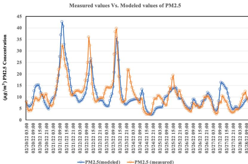
Fig. 7. Comparison of PM2.5 values simulated by CONTAM with measured data.
