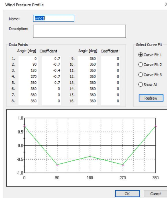
Fig. 3. Wind pressure profile introduced to the CONTAM model.
