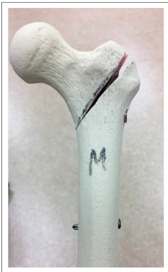
Figure 1. A stable trochanteric fracture model (AO/OTA 31A1.2) was fixed using TFN-ADVANCED Proximal Femoral Nailing System.
