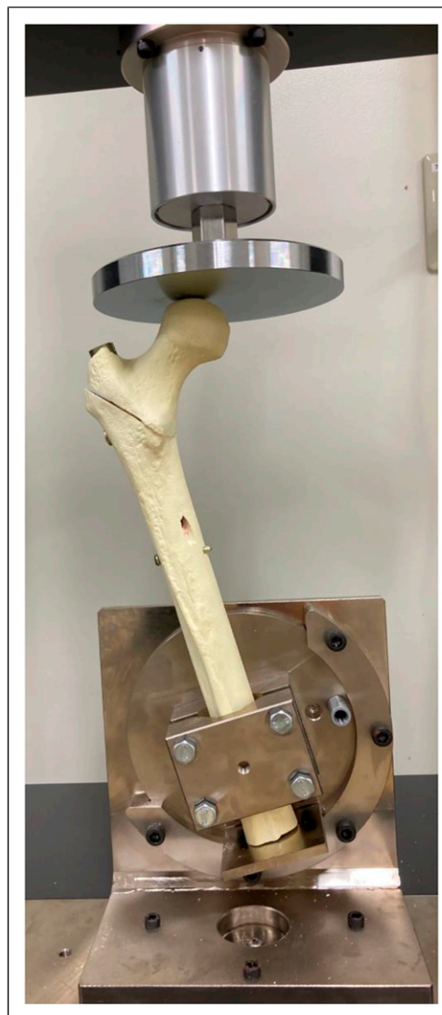
Figure 2. Tensile tester with a set of specially designed grips to hold the distal femur.
