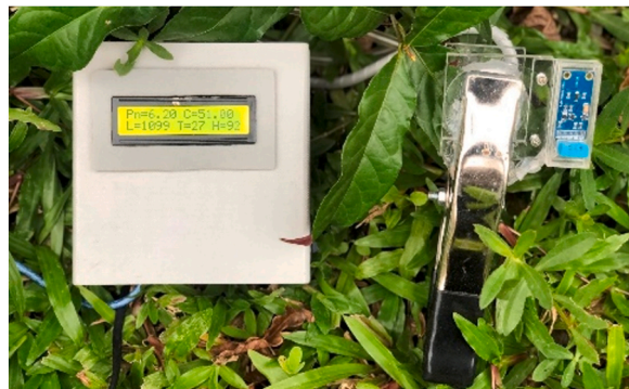
Fig. 4. Advanced photosynthetic sensor.
