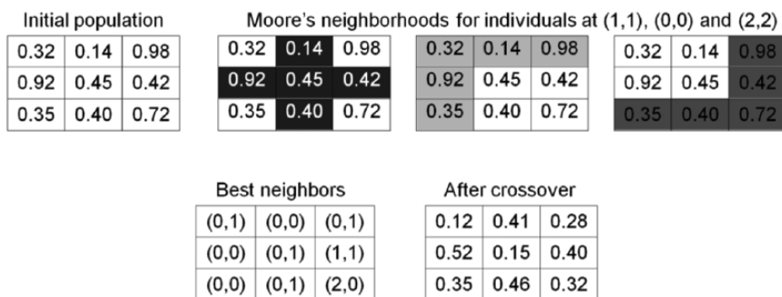
Figure 8. An example showing how the best fitness neighboring element is chosen for each element in a 9-individual cellular population. Top: from left to right, first we depict the fitness value of 9 individuals arranged as a cellular model. On the next 3 diagrams, the Moore neighbors (considering a torus topology) for the individuals situated at (1, 1), (0, 0), and (2, 2) are marked with shadows. Bottom: left, coordinates of the best neighbors for the 9 individuals; right, a possible result after the crossover operation.
