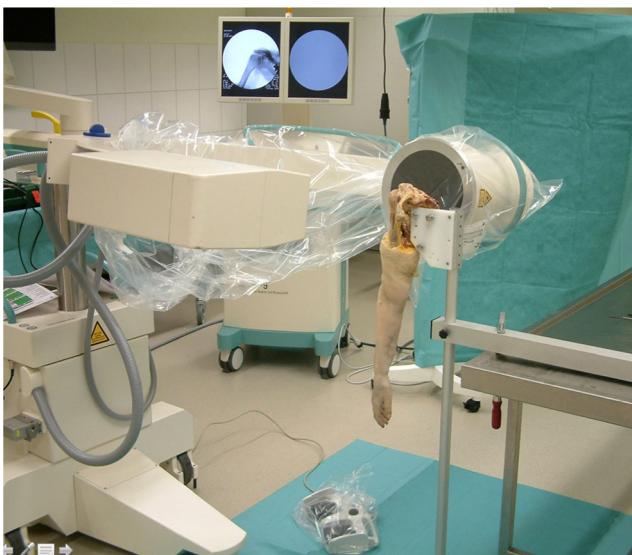
Fig. 4 Photograph showing the experimental setup. The scapula was firmly attached to a special frame in a vertical position
