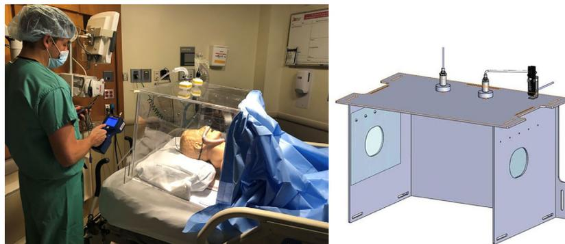
**Figure 1** Photograph and diagram of polycarbonate enclosure with attached wall suction and HEPA filtration. Access holes on the sides were covered with clear plastic flaps and the torso of the simulated patient was covered with an adhesive surgical drape
