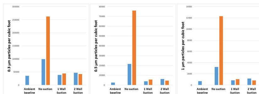
**Figure 2** Number of 0.3, 0.5 and 1 micron particles per cubic foot detected outside the enclosure. Particle counts were measured at baseline, 1 min after (blue) and 5 min after (orange) release inside the enclosure
