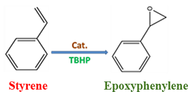
Scheme 2. Oxidation Reaction of Styrene Catalyzed by the Hierarchical LTA Zeolite
