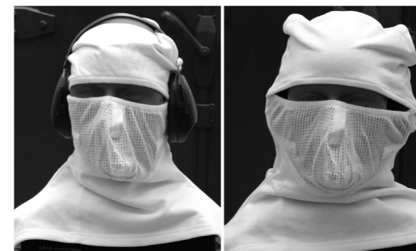
Fig. 4. The Peltor H515FB earmuffs worn over and under the anti-flash hood.
