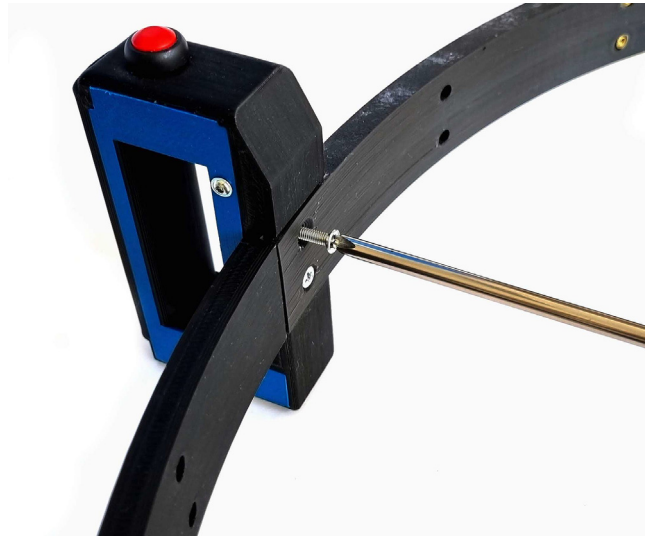
Fig. 14. Assemble two frame parts and one of the grips with two M4*20 mm screws.
