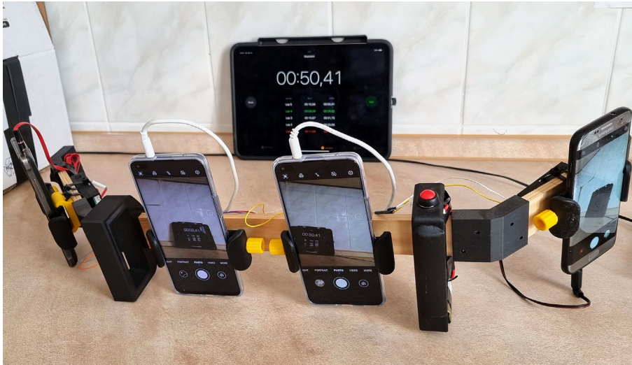
Fig. 17. Testing the release lag between the cameras. The frame is an early prototype, the circuits are as described in the paper.
