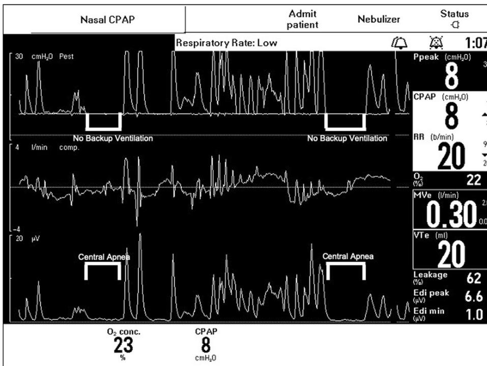
**Fig. 2 Period of apnea when on noninvasive pressure support ventilation.** The bottom line is the Edi signal. The next line up is volume and the third line up is flow. The top line is pressure with the pressure estimate (derived from the Edi signal) superimposed. The patient gets pressure support breaths when both breathing and apneic. These are not synchronized with some breaths autotriggering (a), some occurring during expiration (b), and provides minimal support when apneic (c).
