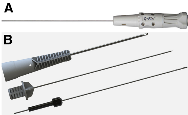
Fig 1. The single-loaded Q-FIX anchor (A) and straight drill guide assembly (B). The 1.8 mm diameter anchor is passed through a 2.0 mm diameter, 22.3 mm length drill hole. (Smith & Nephew Endoscopy.)
