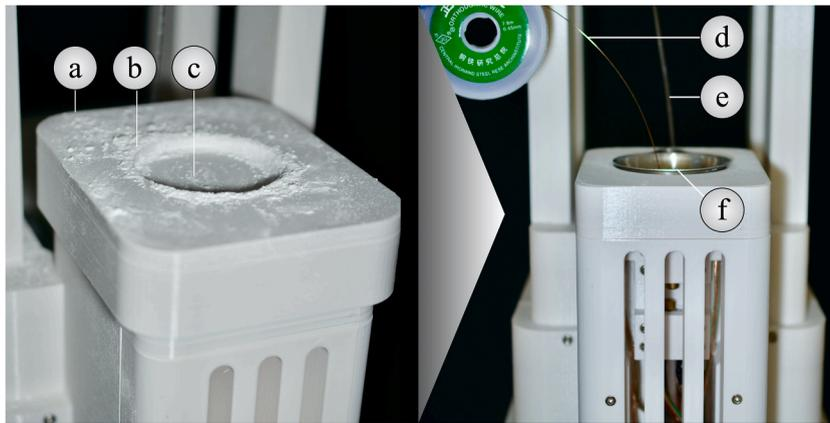
**Fig. 6.** Cleaning of the coating machine for filament
