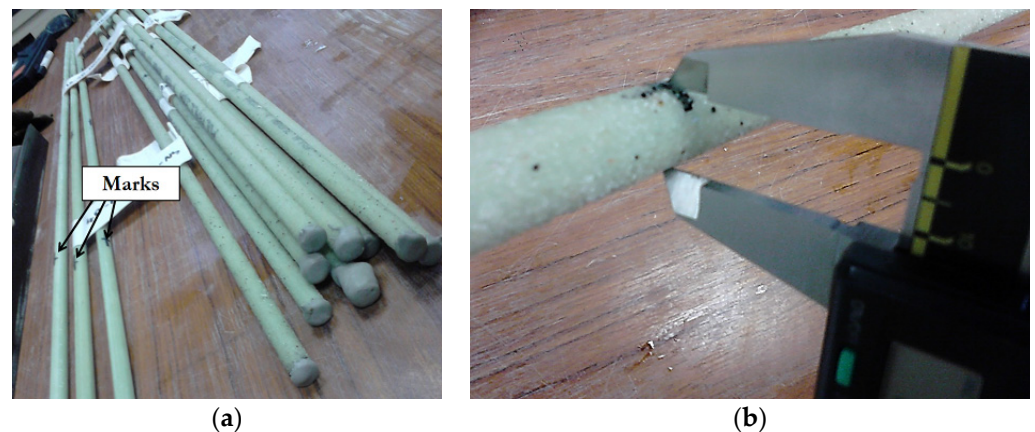
Figure 5. (a) Marked GFRP rebars used for monitoring the changes in mass/diameter over aging and (b) illustration of the diameter measurement on a sand-coated rebar (as a reminder, the nominal diameter of all rebars was 12.7 mm).
