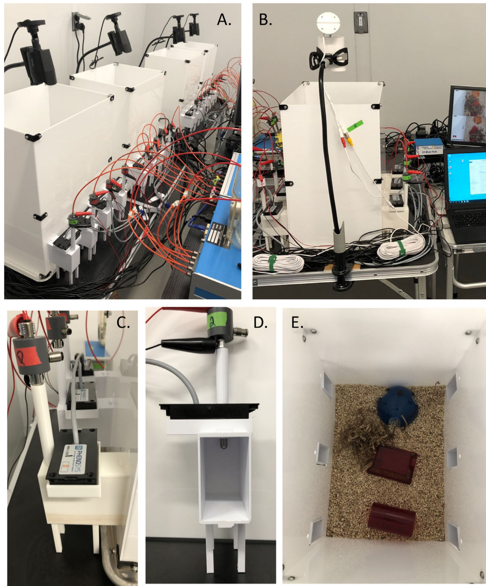
Fig. 2. A) SIT 4-station setup (4 on one side), B) SIT 6-station setup (3 on each side). C) Side view of drinking stations connected to SIT wall; each station includes a 3d-printed cubby, VDM sipper, and RFID sensor. D) Front view of drinking station showing access to tip of sipper tube (metal part that extends into the interior) when the animal is inside the drinking station. E) View of SIT 6-station setup from above.
