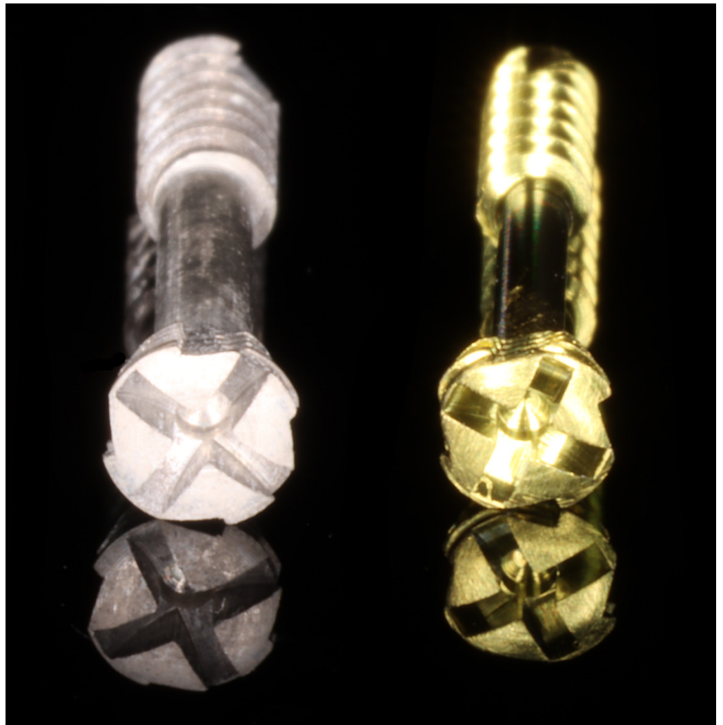
Figure 2. The compression screws used have cross sockets and peripheral notches to collect bone chips. It is assumed that both screw types will be immersed in the bone in their entirety.
