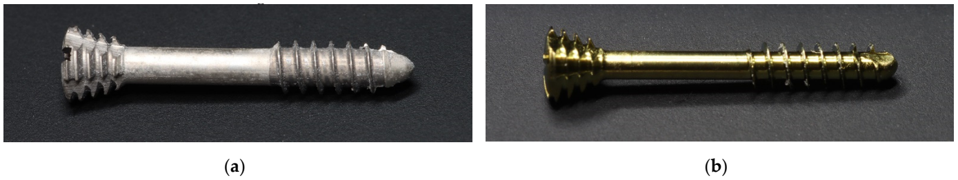
Figure 1. General appearance of the compressive headless screws used in the study. These screws are ChM's dedicated designs for mandibular head fixation. (a) magnesium alloy 2.2 mm screw (test group); (b) titanium alloy 1.7 mm screw (reference group). Compressibility is ensured by different thread pitch. The large pitch at the tip of the screw ensures a large longitudinal movement with every turn in proximal bone fragments. On the other hand, a small thread pitch at the socket end leads to a small longitudinal movement of the screw in distal bone fragments, which ensures a compression effect in the fracture gap.
