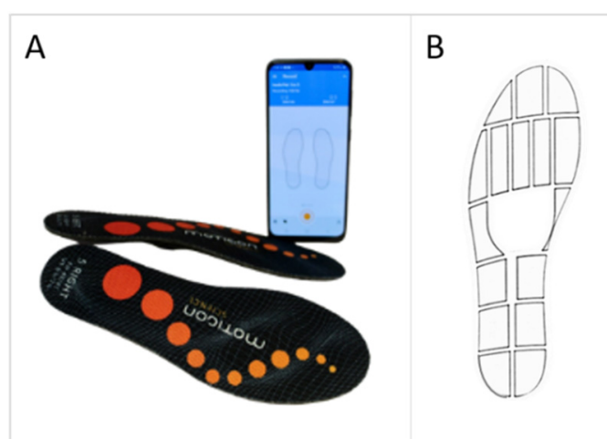
Figure 1. (A) The Insole3 (Moticon ReGo AG, Munich, Germany) and the OpenGo smartphone application. (B) Layout of the 16 pressure sensors and coordinate system. Figure 1B used and modified with permission from Moticon ReGo AG.
