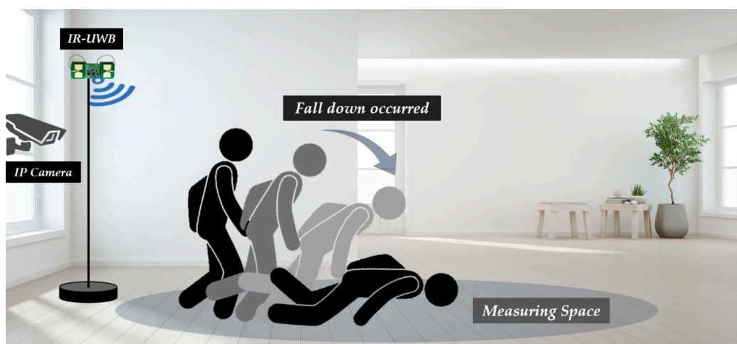
Figure 3. Conceptual drawing of object movement using IR-UWB radar sensor and IP camera.
