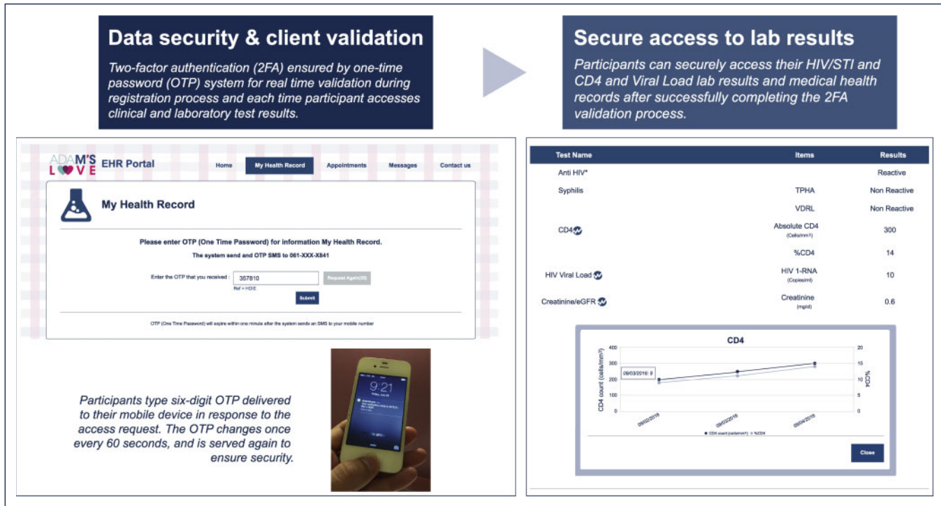
Figure 2. Adam's Love Electronic Health Record (EHR) advanced data security system and one-time password (OTP) verification. Advanced security features included an email verification process and a two-factor authentication (2FA) ensured by an OTP for real-time validation during the registration process and each time participants accessed clinical and laboratory test results
