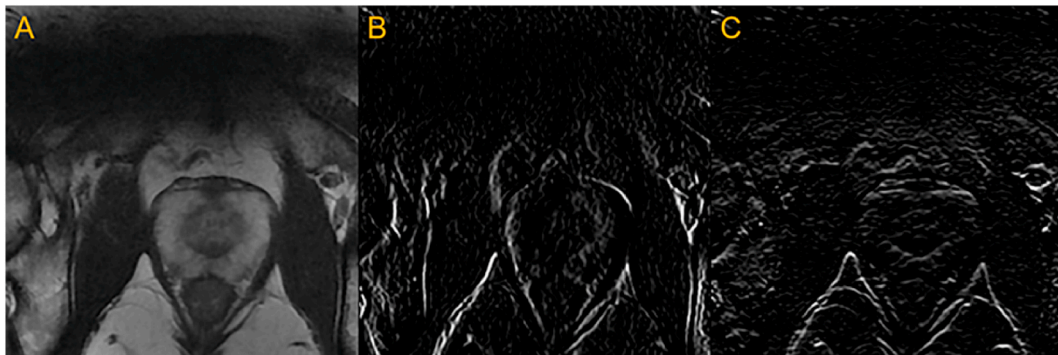
Fig. 7. An example of result image by using the Sobel operator. Notes: A Original diagram, B vertical gradient image, C horizontal gradient image.
