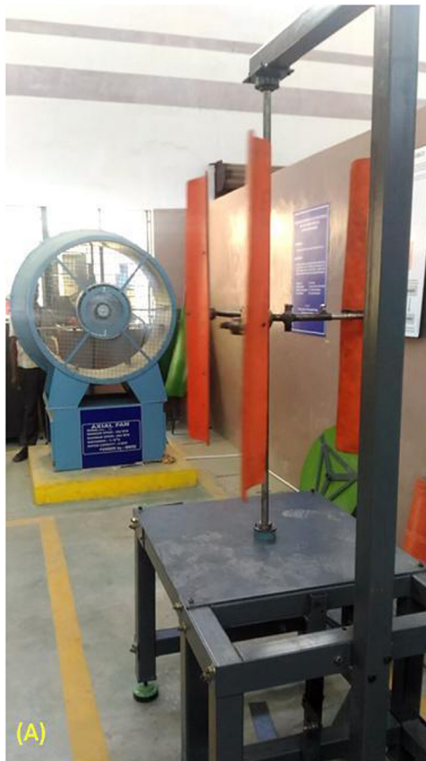
Fig. 1. (a) Experimental setup (b) Close view of the proposed VAWT in test rig.
