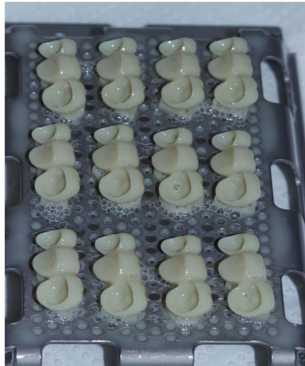
**Fig. 4** A sample of the 3D-printed specimens on the build plate showing the orientation of printing
