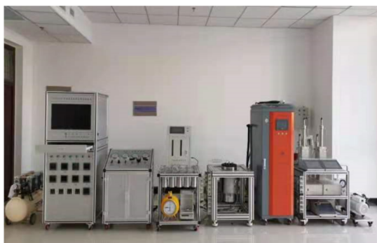
Figure 1. Physical diagram of the gas adsorption–desorption experimental instrument (Photograph courtesy of Yang Wang, Copyright 2022).
