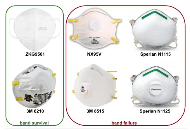
**Figure S4.** Respirators assessed for headband compatibility with ozone disinfection. All of the respirators with failed bands feature stapled attachments.
