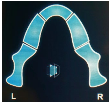
Fig. 4 Image of control panel for OP300 showing five sections for possible selection
