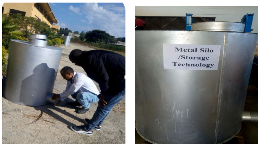
Fig. 1. metal silo cereal storage technology.
