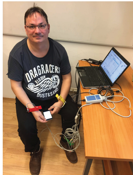
FIGURE 3: Experimental arrangement. The subject is sitting in a resting position, the electrodes of the ECG device are connected to the limbs, and the smartphone is held in the subject’s palm.
