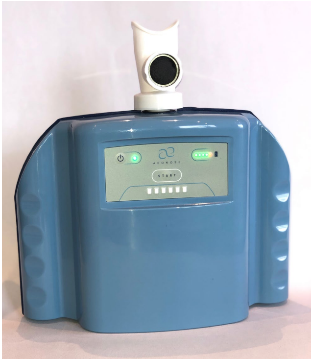
FIGURE 1 Electronic nose used in the study; the Aeonose (The eNose Company). Patients inhale through a carbon filter to prevent the entry of nonfiltered environmental air and breathe into the device through a disposable mouthpiece while wearing a nose clip
