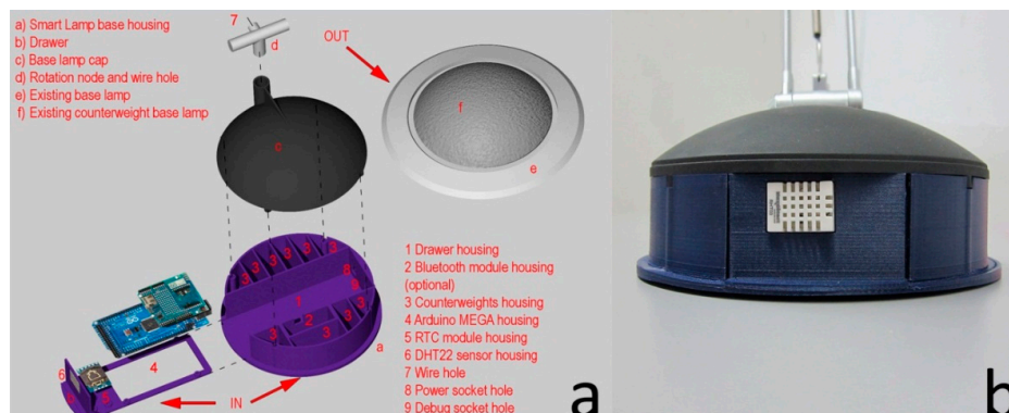
Figure 3. Smart Lamp: (a) assembly diagram of the base; (b) as installed.
