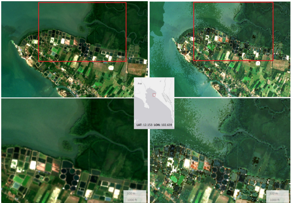
Fig. 6. Trat province of Thailand, January 2019 true colour composite at 10 m resolution (overview and zoom) as computed in GEE using L2A median value (left) and by S2GM using L2A Medoid/STC algorithm (right).
