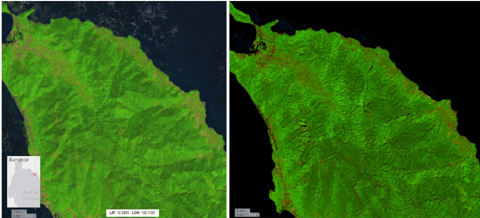
Fig. 5. Ko Chang Island, Thailand, Sentinel-2 L1C TOA reflectance 2019 annual median composite processed in GEE (left) and overcorrection of north-facing slopes as obtained from S2GM 2019 annual composite (right) using the L2A BOA reflectance products. Both images are displayed in false colour composite (SWIR1, NIR, RED).
