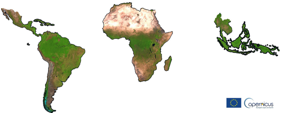
Fig. 1. Extent of the proposed annual Sentinel-2 L1C cloud-free composites. False colour combination (SWIR1,NIR,RED) of year 2020 median layer.
