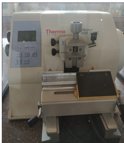
Figure 2: Semi-automatic soft tissue microtome
